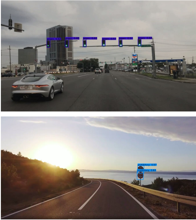
Fig. 4. Examples of YOLOv4 tiny detection and recognition.
