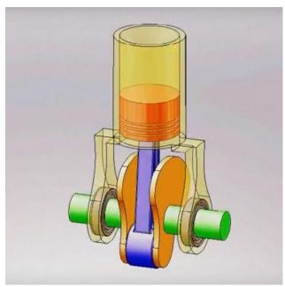
**Slider-crank chain inversion** arises when the connecting rod, or coupler, of a -crank linkage becomes the ground link, so the slider is connected directly to the crank
