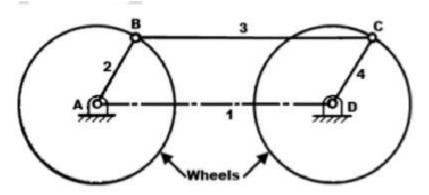
Links -links AD frame (Fixed), link AB (Crank), link BC (Coupling Rod), link CD (Crank) Pairs -Turning Pair = AD (Frame) & AD (Crank), Turning Pair = AD (Frame) & CD (Crank), Turning Pair = AB (Crank) & BC (Connecting Rod), Turning Pair = CD (Crank) & BC (Connecting Rod)
